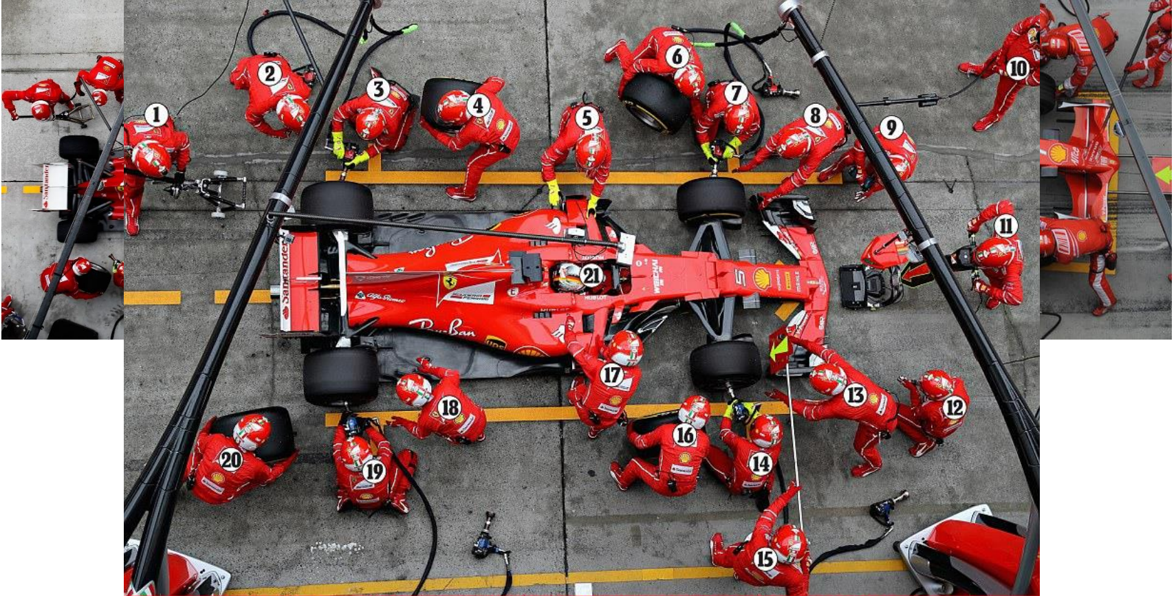
1. Rear Jack 2. Rear Tyre Off 3. Tyre Gunner 4. Rear Tyre On 5. Stabiliser 6. Front Tyre On 7. Tyre Gunner 8. Front Tyre Off/Stop Marker 9. Front Wing Adjuster 10. Backup Front Jack 11. Front Jack 12. Front Wing Adjuster 13. Front Tyre Off / Stop Marker 14. Tyre Gunner 15. Lollipop Man 16. Front Tyre On 17. Stabiliser 18. Rear Tyre Off 19. Tyre Gunner 20. Rear Tyre On 21. Driver
